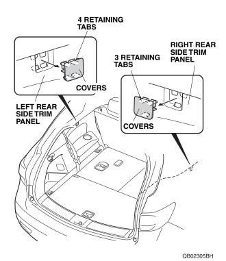
9. Install the cargo cover into the recess in the right rear side trim panel, then compress the cargo cover, and install it in the left rear side trim panel.
